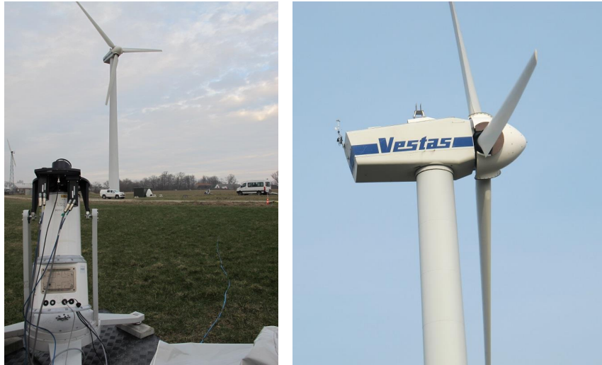
Figure A.2: Lidar 2 positioned in the field with V27 wind turbine in the background (left). Close-up of V27 nacelle and rotor (right).
