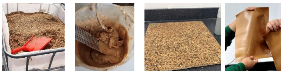
Fig. 3. Brewery spent grain used to create bio resin, bio board and bio leather (Source: Authors)
