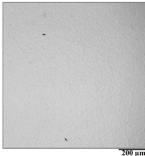
Fig. A1. Example image used to analyse the pores (the dark spots) found in the microstructure of Ti64.
