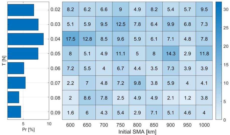
Fig. 20 Matrix of the probabilities of permanent capture into 1:1 GTR for different thrust magnitude values and initial semimajor axis. On the left, is a histogram of the mean value of the probability of permanent capture into GTR for each thrust magnitude value
