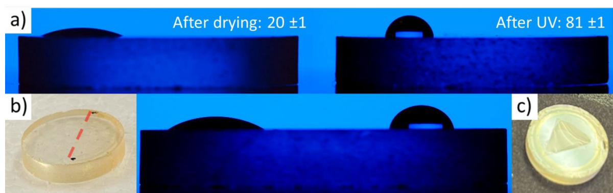
Figure 5: a) Example contact angle measurement of a thin film of 7-OH before (left) and after (right) 365 nm LED irradiation. b) Example of the contact angle change in a single film of 9-OH, where half the film has been irradiated while the other half has been covered with a photomask. The red line in the picture (left) represents the location of the photomask, which gives rise to the change in the water droplet contact angle (right) on the same substrate. c) Picture of how different photomasks can be used to control the surface wettability, herein a triangle shape photomask.
