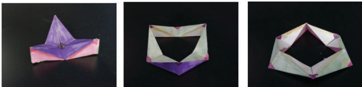
Figure 4.34 Paper model of an ‘invertible cube’ or ‘Schatz cube’ in various motion states
