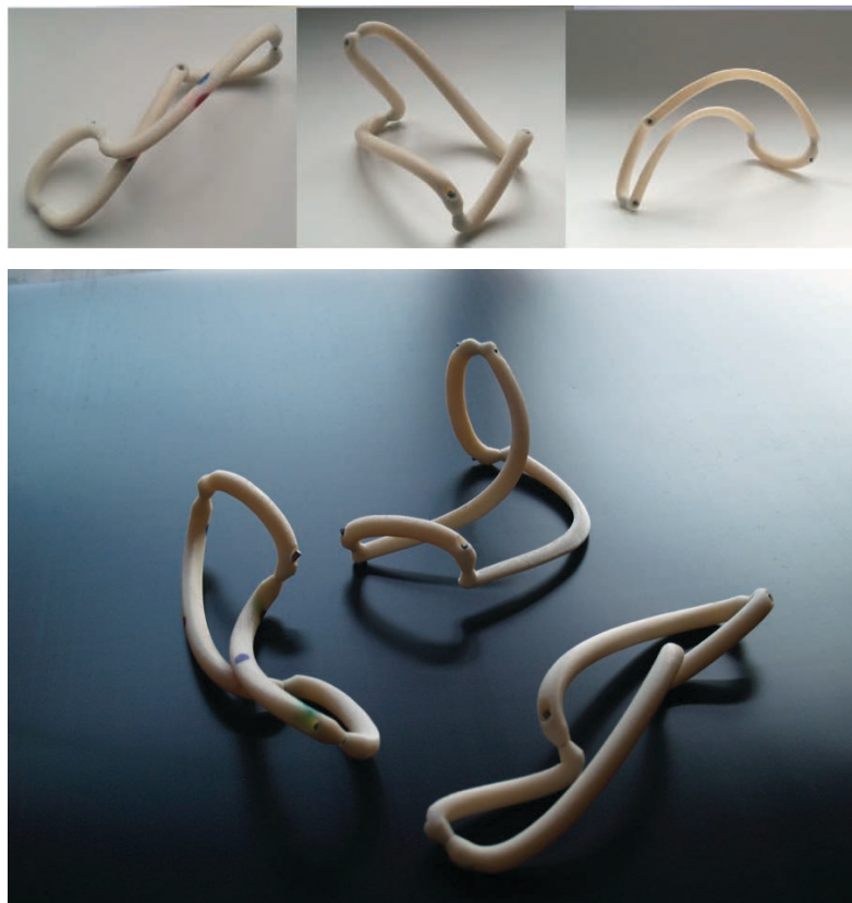
Figure 4.39 3D printed models of 4 bar Bennett linkage, showing 3 possible instantiations (two of which exhibit successful full cycle motion)
