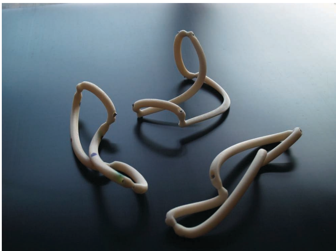
Figure 2.4 3d-printed models of over-constrained linkages (Harrison et al., 2011)
