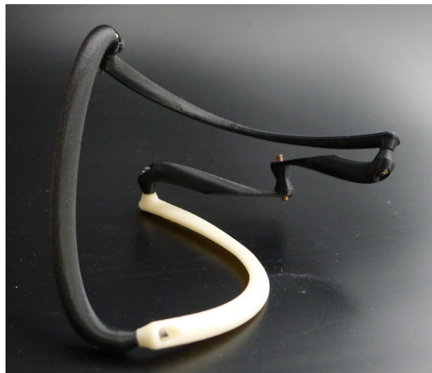
Figure 4.46 Bars from previously fabricated models were reused, with sites of interference cut away
