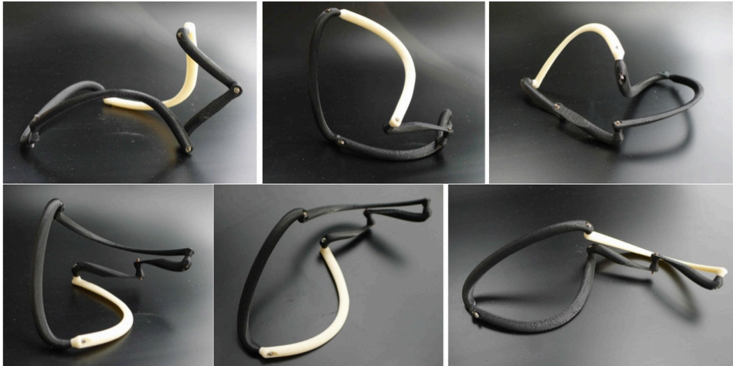
Figure 4.45 Goldberg Five-bar linkage
