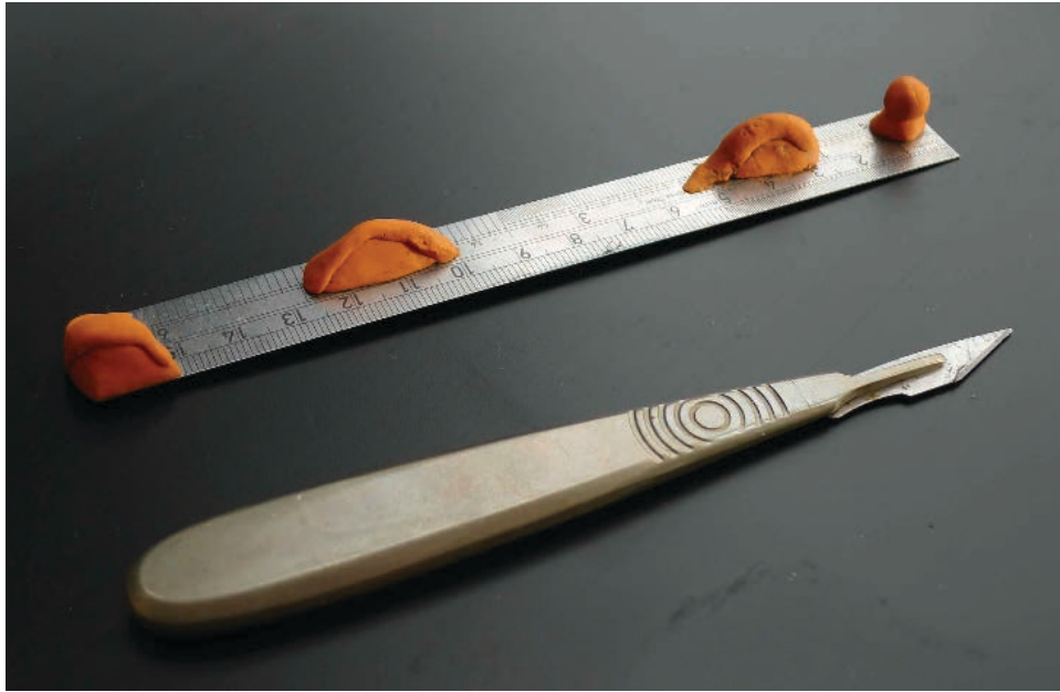
Figure 4.5 Tools used in many of the making examples. Rubber handles (orange) augment the ruler to help repositioning
