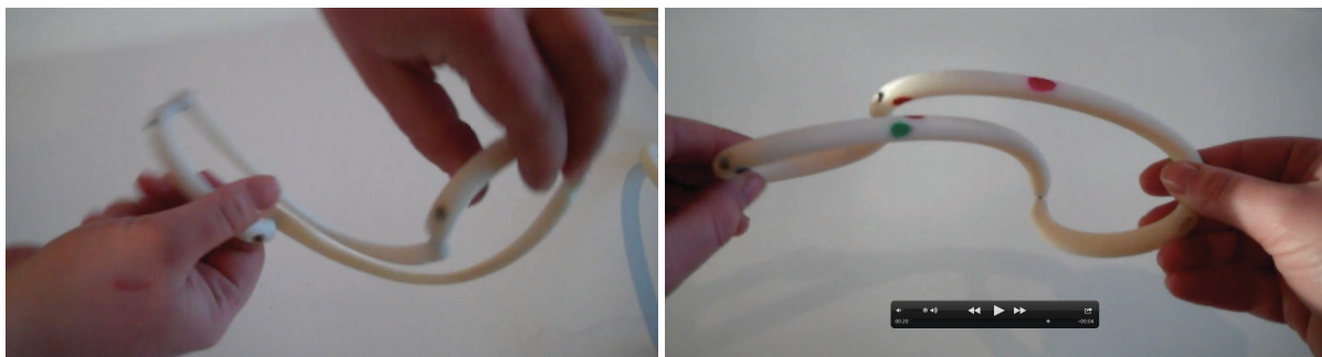
Figure 4.49 Manipulating 3d-printed models of over-constrained linkages (Harrison et al. (2015) has a video link)
