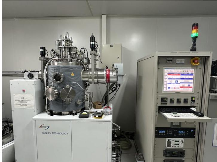
**Figure 3.4 Magnetron sputtering equipment.**
