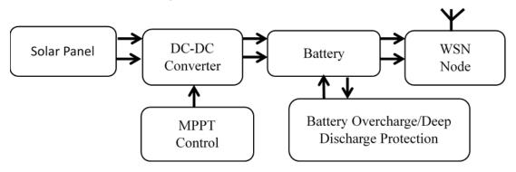
Fig. 4. A block diagram of solar energy harvesting mechanism [41]
