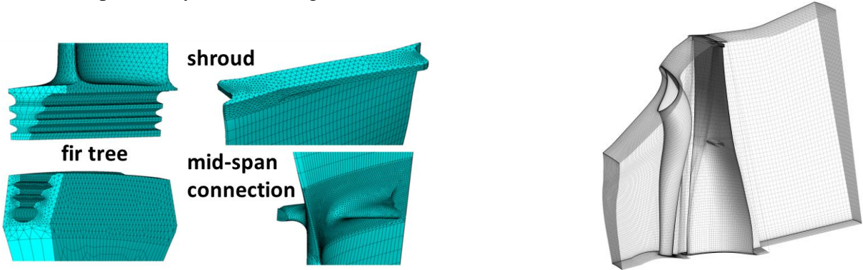
Fig. 3. Details of the structural model parts (left), CFD mesh (right)
