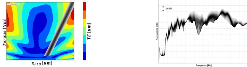
Fig. 7. (a) Load path distribution together with probability distribution of the gear tilting (b) An example illustrating the propagation of system response-induced structure-borne noise, assessed within coupling positions to the car frame, arising from variations in gear mesh excitation
