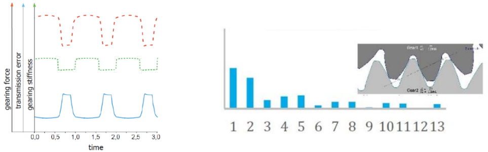
Fig. 4. (a) Example of periodic gear mesh excitation (b) Fourier coefficients
