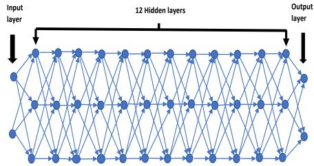
Figure 2. Feedforward Artificial Neural Network (ANN): input layer, 12 hidden layers with three neurons for each layer, and output layer
