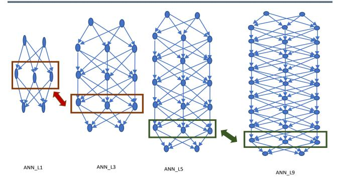
Figure 5. Crossover operation between the top 4 ANN layers in layers
