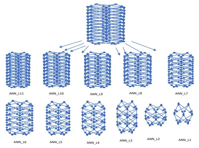
Figure 3. The main ANN (12 layers) breaks into 11 ANN from left to right: 11 layers, 10 layers, 9 layers, 8 layers, 7 layers, 6 layers, 7 layers, 6 layers, 5 layers, 4 layers, 3 layers, 2 layers, and 1 layer
