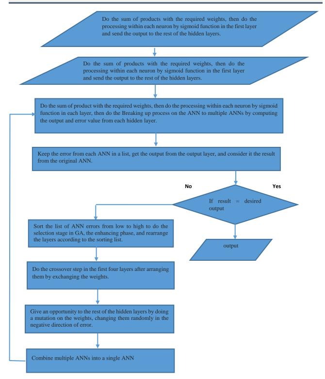
Figure 1. The flowchart of the neuro-genetic model
