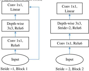
Figure 3. MobileNet-V2 architecture.
