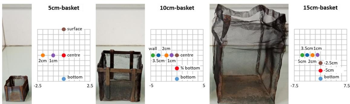
Figure 2: Spatial distribution of thermocouples for the three basket sizes
