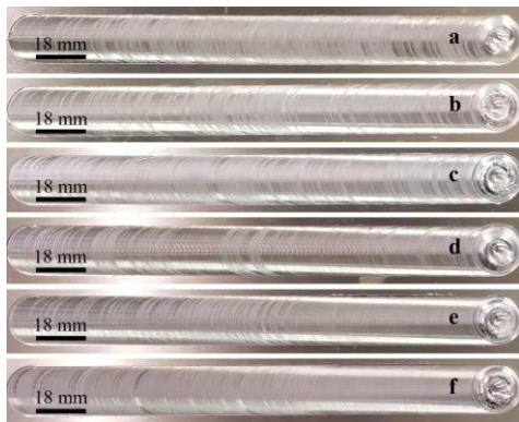
Fig. 3. Surface appearance of the WJs under different process parameters: a–GN 1; b–GN 2, c–GN 3; d–GN 4; e–GN 5; f–GN 6
