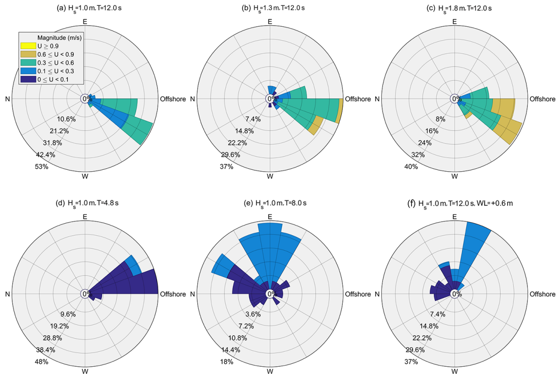
Figure 5. Rip current rose diagrams of rip currents forced by different wave conditions and tidal levels at positions x = 730 m and y = 120 m marked as Gauge A in Fig. 1f. Each spoke denotes the direction that the current flows to. The offshore direction is labeled in each diagram. T1 and T7–T8 are not included.
