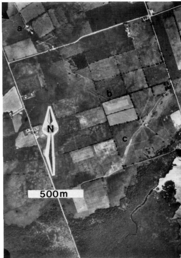
FIGURE 10. Aerial photograph of Cawker-Williams pop-up set. Note locations of a) trench; b) pop-ups (between arrows); c) Lake Algonquin paleobeach. Note the barn on the intersection of a pop-up and the paleobeach.
