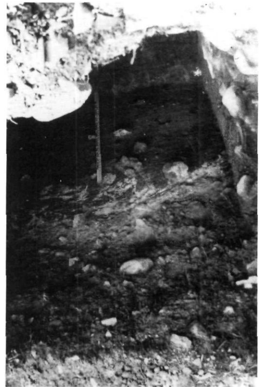
FIGURE 4. Test trench to bedrock, showing disturbance of proglacial lake clays (above yardstick) and overlying till.
