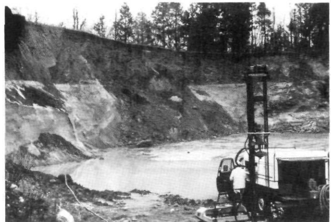
FIGURE 5. Exposed section of the west end of the Bélanger pit in mid-November 1982. The drill is at borehole 5. Note planar contact between the upper till (unit 6) and the unfossiliferous sand (unit 5), GSC photo No. 203990-G.
