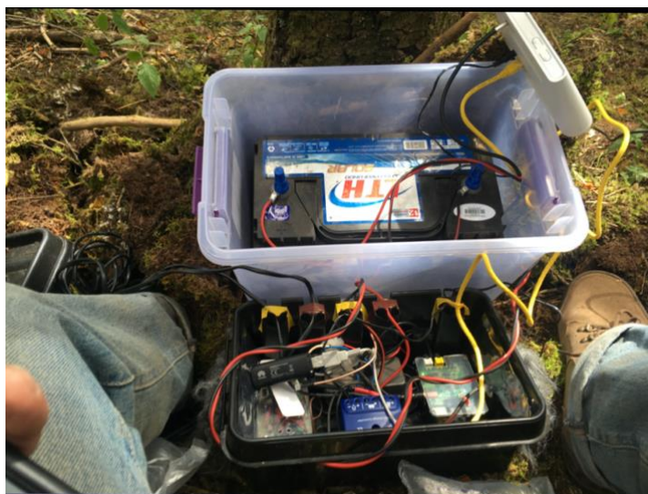
Figure 2. Streambox and battery with wireless router in the Cerro Pelón UNESCO Biosphere Reserve in the State of Mexico.
