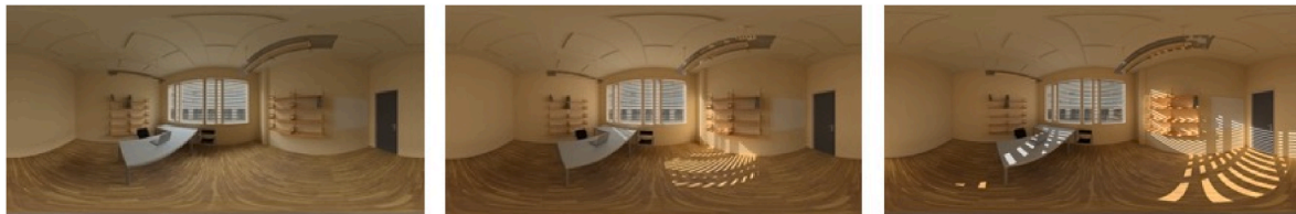
Fig. 10. Rendering of a space from the Chamilothoni dataset lit by three sky conditions: overcast (left), clear sky with high sun position (center), and clear sky with low sun position (right).
