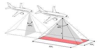
Fig. 3. FOV relation to the (AOV) and altitude h [14]
