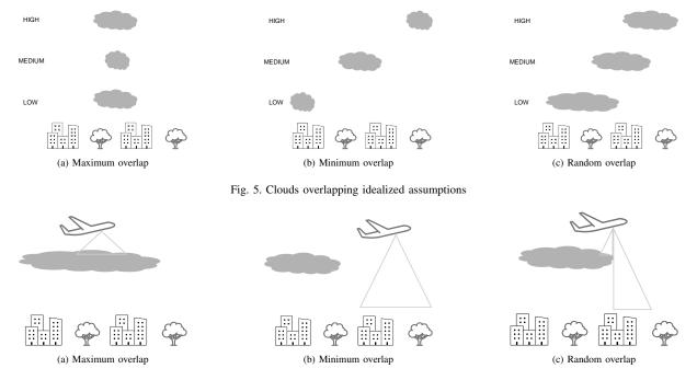
Fig. 6.  $FOV_h$  of camera mounted on the aircraft and clouds overlapping idealized assumptions
