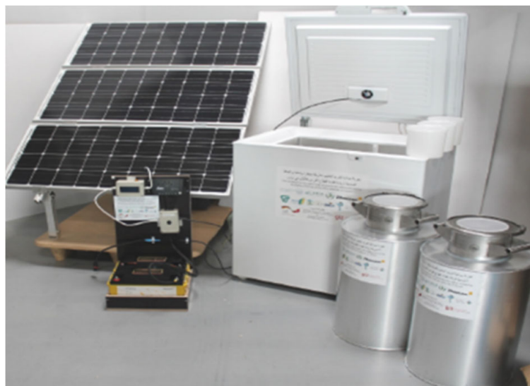
Figure 4. Solar-powered milk cooling innovation developed by Hohenheim University (PV panels, 2 batteries, control panel, solar freezer, 25 ice blocks, and 2 milk cans) [37].
