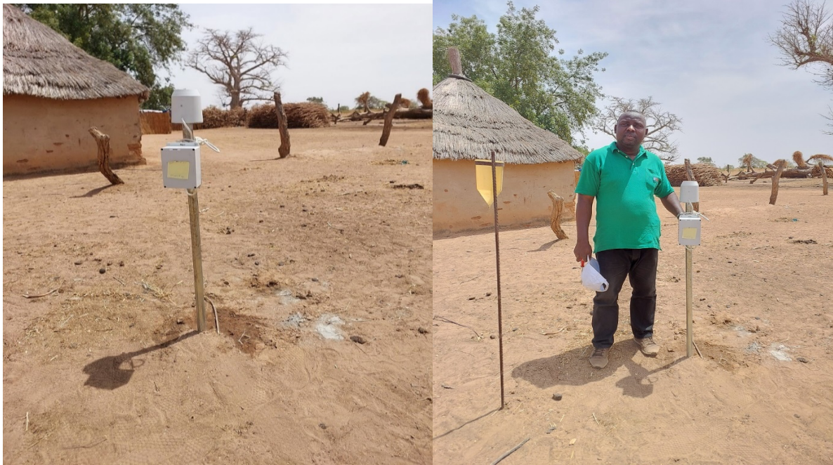
Photo 8: Installation of both IoT and Manual Rain gauges at Bousra village in Koumpentum cluster, Tambacounda region.
