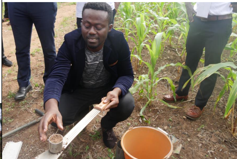
Figure 5: Soil sampling during the practical session at the Soil Science experimental fields, KNUST, Kumasi
