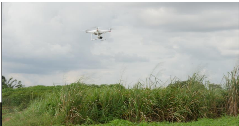
Figure 8: Drone taking spatial data during the practical session at the Soil Science experimental fields, KNUST, Kumasi
