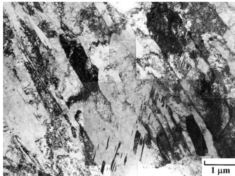
Figure 2. Cast TEM imaging of the martensite microstructure [13].
