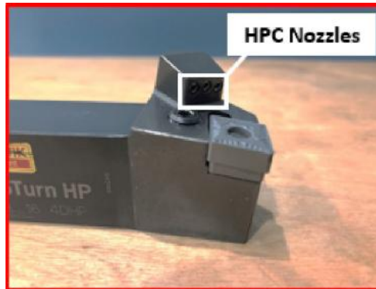
Figure 7: View of cutting tool holder with high pressure coolant Nozzles (Stolf et al. 2019)
