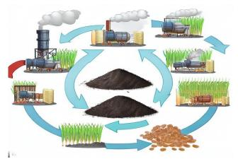
Figure 3. Scheme of Biochar production from crops
