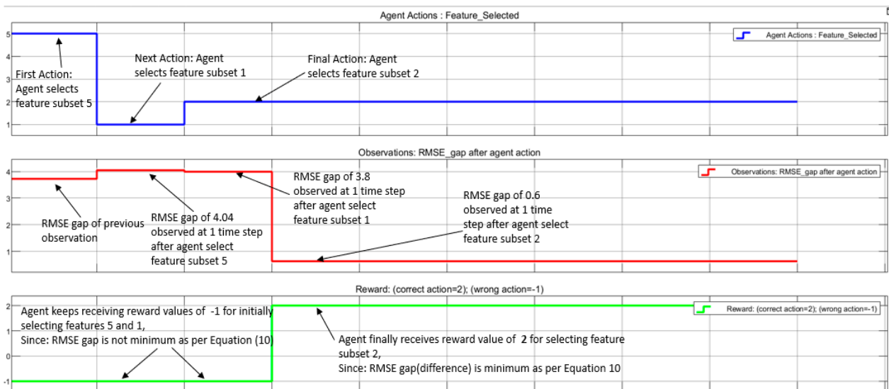
Figure 17. Plot from DRL model showing agent actions (in blue), current/previous RMSE (red), and rewards (green).
