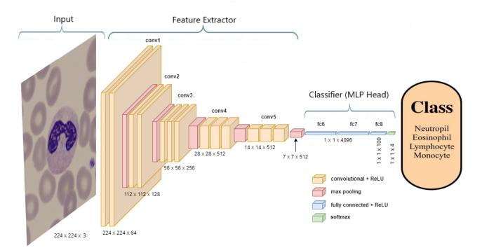
Figure 4. Architecture of VGG-16 model classifying a neutrophil.
