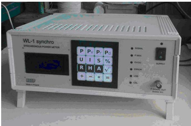
Fig. 2. WL-1 synchronous power processor.
