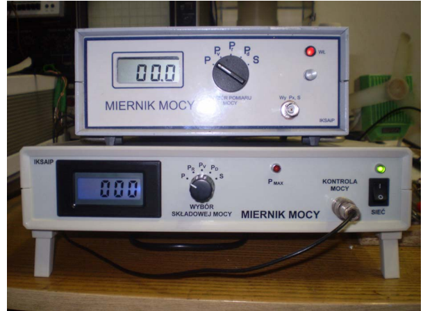
Fig. 3. Power meters (voltage and current measurement terminals on the back of the instrument).
