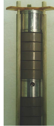
Fig. 3. Varistor column with inserted temperature logger
