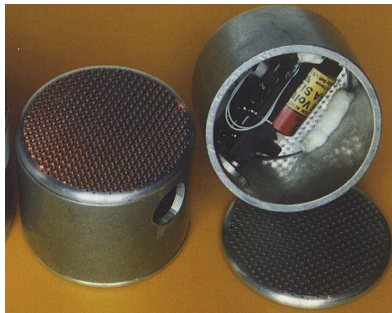
Fig. 2. TINYTALK temperature sensor integrated in a Aluminium tube
