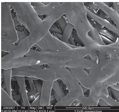
Figure 9. Microscopic image (SEM 1000x) of the surface of a sputtered Zn-Bi sample.
