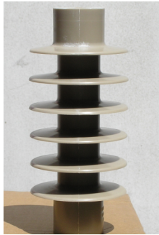
Fig. 1. The insulator made from HCEP
