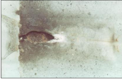
Figure 6. Surface erosion of tested samples,
