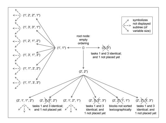
Figure 4: Generation of branch-and-bound tree and symmetry breaking.
