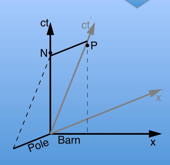
In the barn's reference frame, the pole will contract and will fit into the barn. In the Flash's reference frame, the backdoor opens (event P) before the front door closes (event N) so he crosses the barn without bumping into the backdoor.
