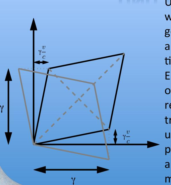
Using the two dashed lines, which represent right- and left-going light pulses, we find how a moving observer's space and time axes deform. According to Einstein's postulate-the speed of light is the same in any reference frame-light must travel one x unit in one time unit. So, the dark (light) parallelogram represents an allowed unit cell of an observer moving to the right (left).
