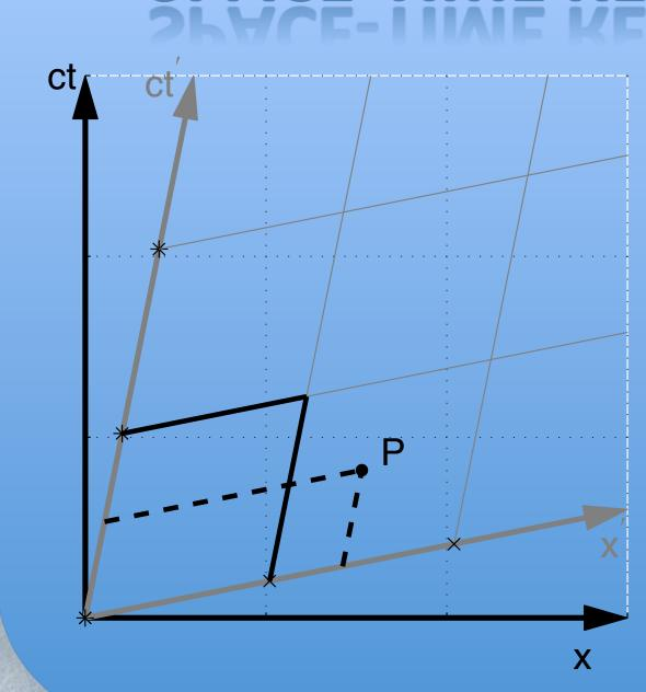
A point P is represented differently in two reference frames. In observer 1's reference frame (dark axes), x and ct are simply the Cartesian projections of P. Observer 2's x' and ct' coordinates are obtained by the projection indicated with the dashed lines.
