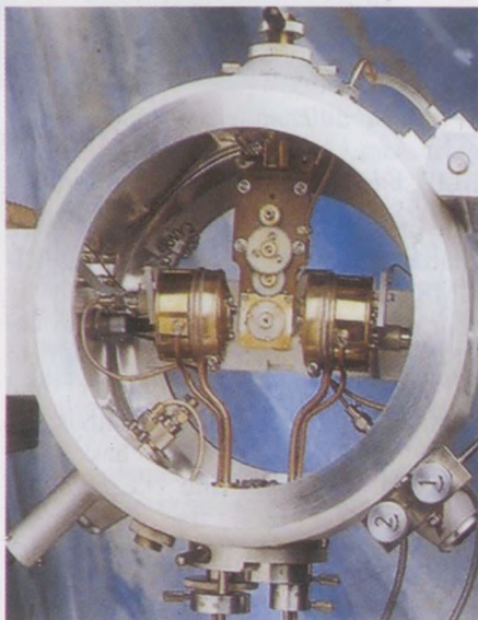
Extreme low-energy ion gun for artifact-free surface layer removal
