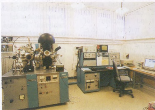
Kratos XSAM-800 type X-ray photoelectron spectroscopic (XPS, ESCA) instrument Research laboratory Materials and Environmental Chemistry, Chemical Research Center
