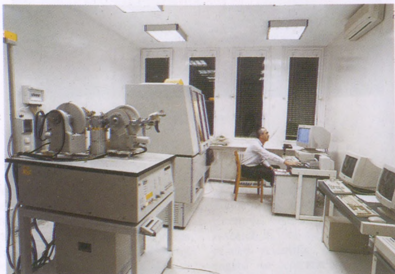
X-ray laboratory for structural studies of polycrystalline and amorphous materials Institute of Chemistry, Chemical Research Center
