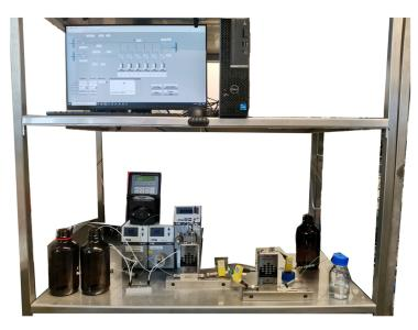
Figure 26. Set-up of the mixing section for the LNP formulation.
