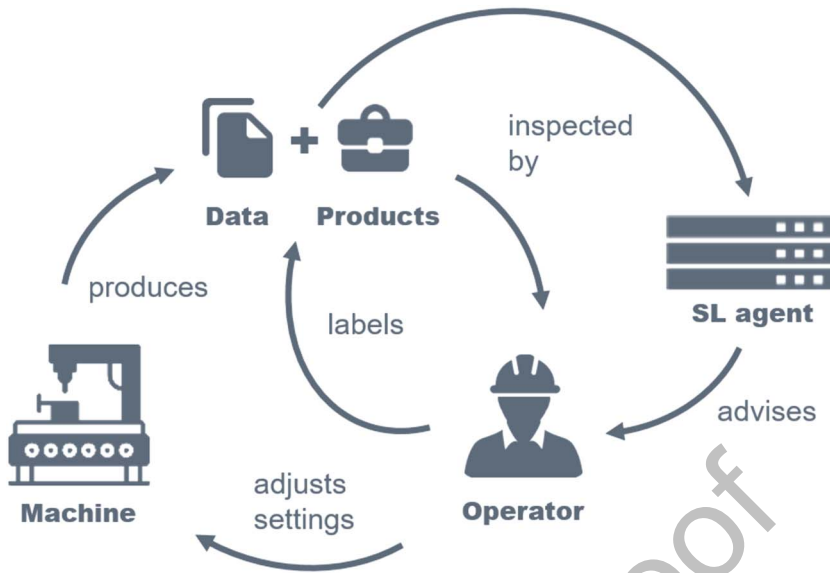
Figure 2. Assisted production using an agent trained with supervised learning (SL) during operation.
