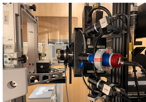
Fig. 1. A schematic representation of the system is presented in panel (a). The projector P_1 illuminates the scene with a Ronchi pattern. The deformation of this pattern is visible on the images acquires by two sensors S_1 and S_2 . The other system’s unit ( P_2 , S_3 and S_4 ) is mirrored on the opposite side of the Z axis. In panel (b) our actual setup is shown. The right-hand side optical unit ( P_2 , S_3 and S_4 ) is visible.
