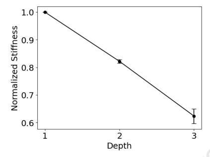
**Figure 5:** The stiffness calculated based on the exponential fit at each depth was normalized with respect to the stiffness of the anterior layer. This normalized stiffness ratio showed a linearly decreasing stiffness from the anterior to the posterior part of the cornea.
