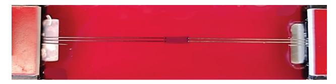
**Figure 2:** The corneal strip (6 x 2 x 0.15 mm) was tested under traction in a bath of MEM + 5% dextran with BioRake attachments. Note that one of the tins has been cut on both sides to leave only two for sample attachment.
