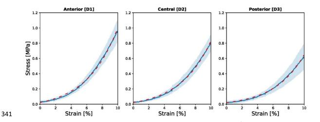
**Figure 3:** The Stress-Strain reaction of the strips in the anterior (D1, n=7), central (D2, n=8) and posterior (D3, n=8) groups. The solid blue line represents the mean stress, and the shaded region represents the standard deviation. The dashed red line represents the exponential fit with equation 1.
