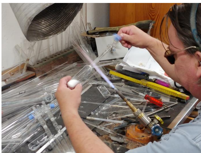
Figure 11. Mr. Müller from Glasbläserei Müller (Adlershof, Berlin) closing ampules with a hydrogen flame of a reaction mixture for graphitic carbon nitride synthesis.
