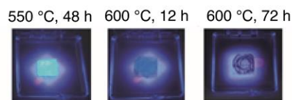
Figure 35. Illumination of PTI-LiBr samples from different reaction conditions with a 375 nm LED. The sample obtained at 550 °C shows visible photoluminescence. Figure adapted from Burmeister et al.. [115]
