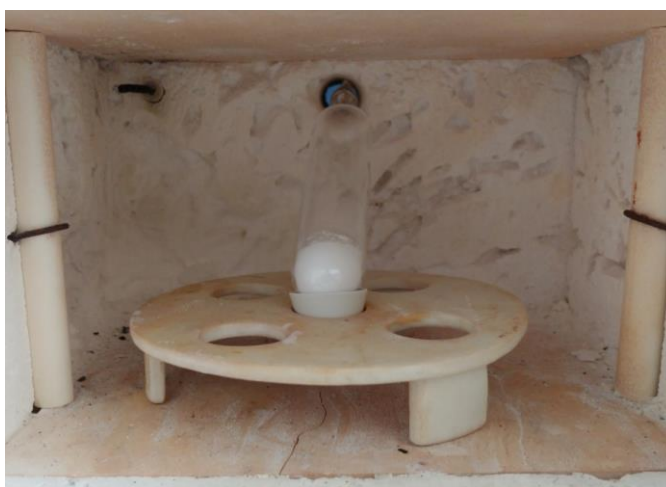
Figure 12. Additional porcelain spacers between bottom plate and ampule to reduce over-shooting the target temperature during heating slopes.
