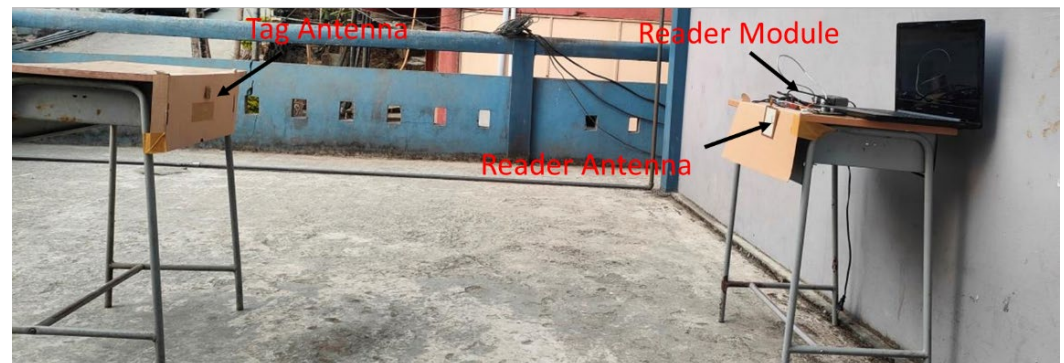
Figure 11. Measurement setup for read range in the free space for maximum distance.
