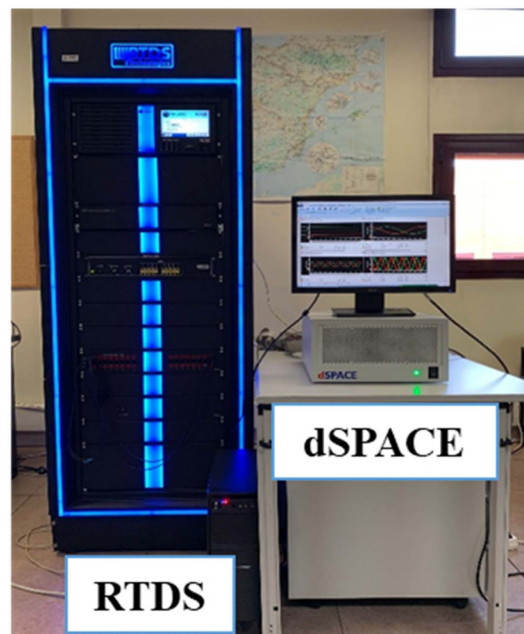
Figure 14. Hardware in the loop experimental set-up.
