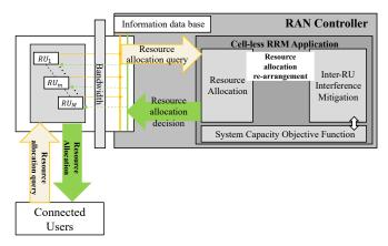
Fig. 1: System model with RRM application within cell-less RAN architecture.
