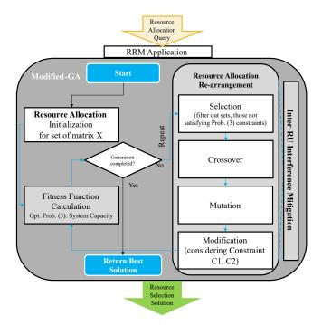
Fig. 2: Flowchart of the modified genetic algorithm (MGA) for cell-less RRM application.
