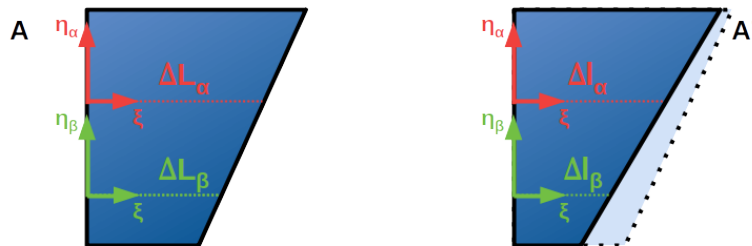
Figure 4. Block's energy invariance under change of reference material line. A : In red is represented the reference frame \xi - 0 - \eta_\alpha integral with the block, when the reference material segment is placed at an height \alpha h from the block's bottom surface. The length of the reference segment is \Delta L_\alpha . When the reference material segment is placed at a different height \beta h , the corresponding frame \xi - 0 - \eta_\beta is depicted in green and its size is \Delta L_\beta . A' : The block undergoes a deformation from its natural shape (light blue): the size of the reference fiber changes to \Delta l_\alpha or \Delta l_\beta . The energy cost associated to this deformation is the same whether the reference segment is placed at \alpha h or \beta h .
