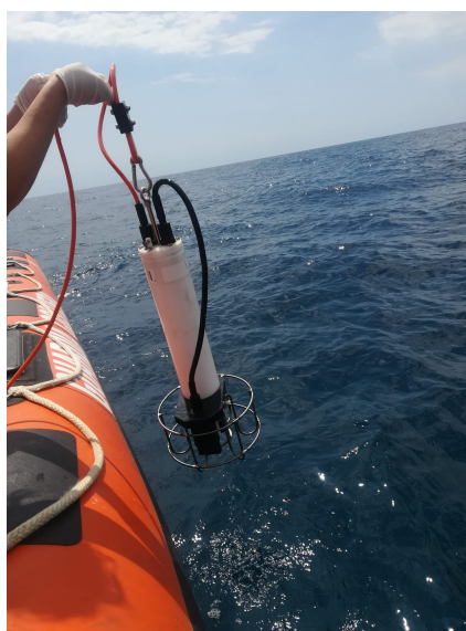
Figure 3.6: Turbidity measurements by a turbidimeter mounted on a submersible probe.
