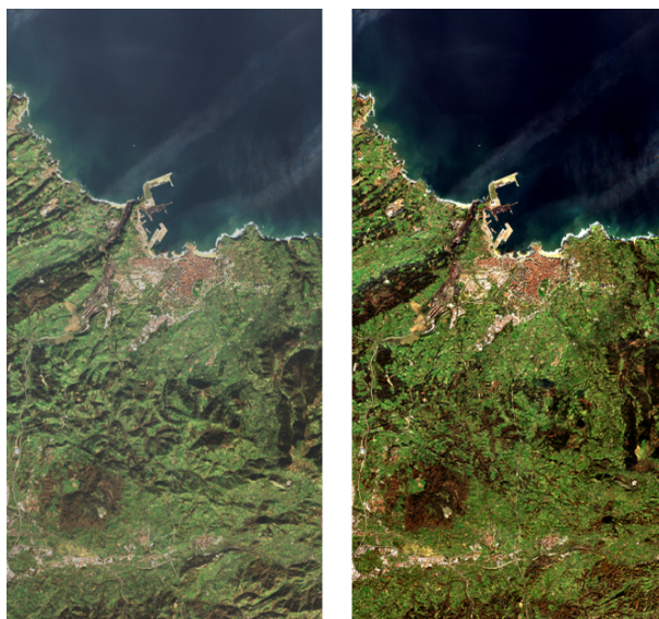
Figure 1.5: A True Color Image obtained from Sentinel-2 MSI Level-1C (left) and Level-2 (right) products.
