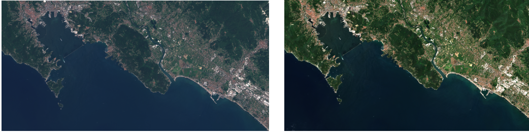
Figure 3.10: Comparison of a True Color Image in the study area obtained from Level-1C (left image) and Level-2A (right image) Sentinel-2 MSI products.
