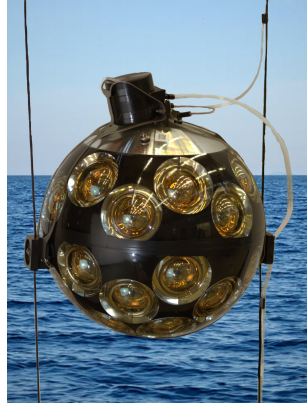
Figure 2.8: Picture of the KM3NeT DOM fixed on the two parallel Dyneema ® ropes. This picture is taken from the KM3NeT official website, https://www.km3net.org/ .
