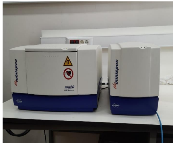
Figure 1. Photo of Bruker Minispec mq20 TD-NMR device(20MHz)
