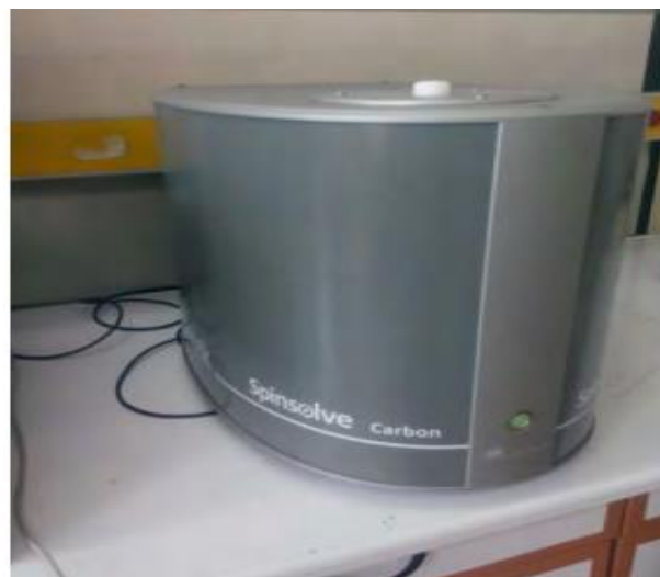
Figure 2. Photo of Magritek Spinsolve NMR spectrometer (42MHz)
