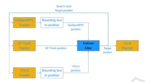
Figure 3: Scheme of our tracker-fusion method.
